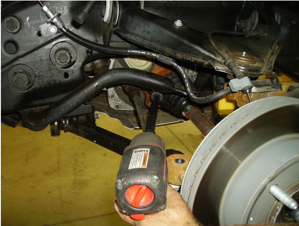
Figure 8: Remove CV axles on 4wd vehicles
