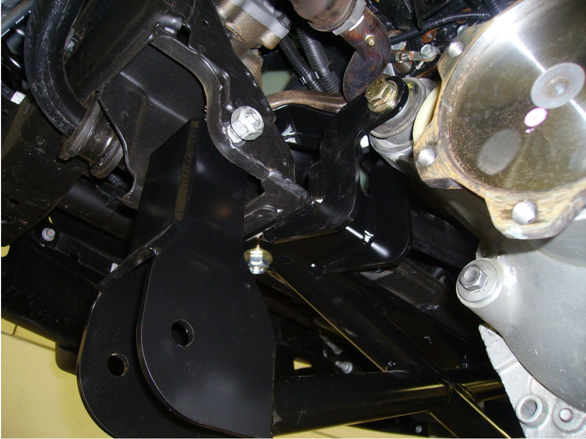
Figure 19: Front xmb and top mount on differential.
