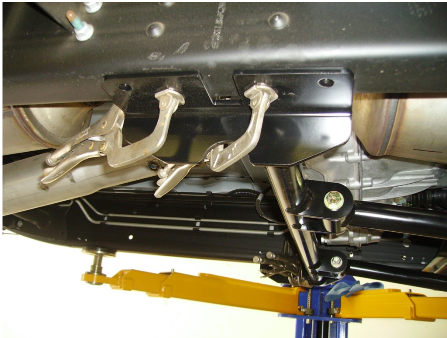
Figure 23: attach 8056 crossmember to 8053 compression strut tubes.
