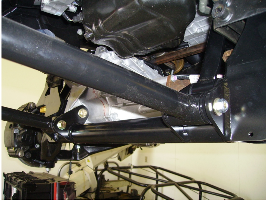
Figure 22: Attach 8033 compression strut tubes to 8071 crossmember
