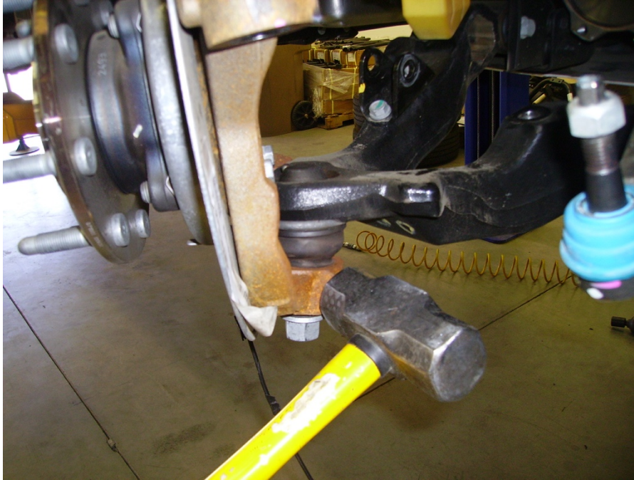
Figure 9: removing lower control arm.
