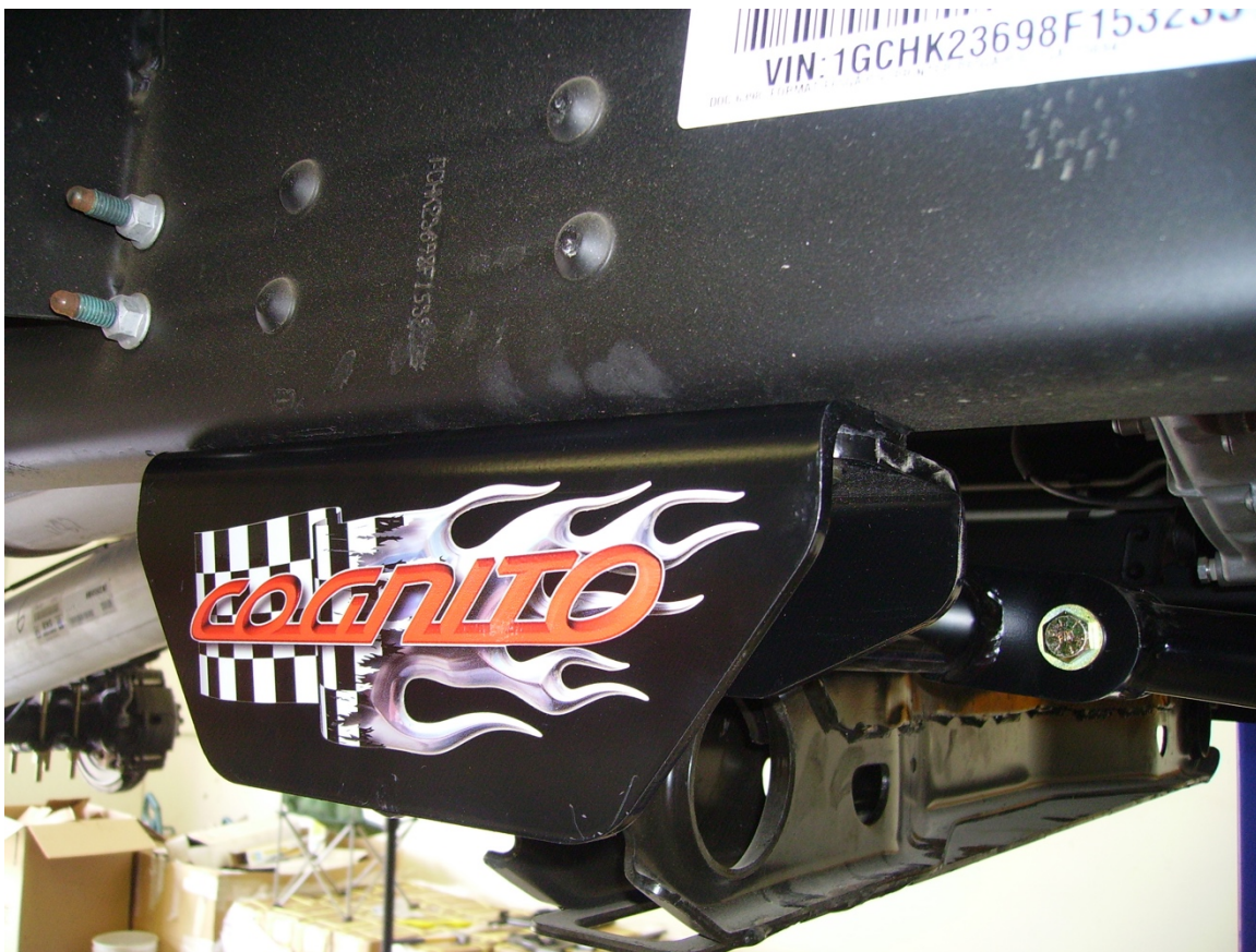
Figure 24: mounting the 8076 torsion bar brackets
