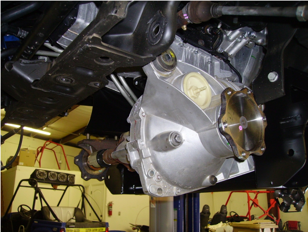
Figure 18: Differential mounted to 8071 and 8072.
