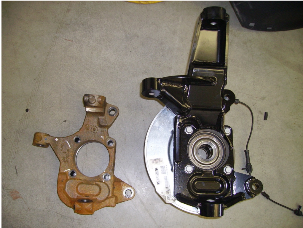
Figure 20: spindle assembly, passenger side
