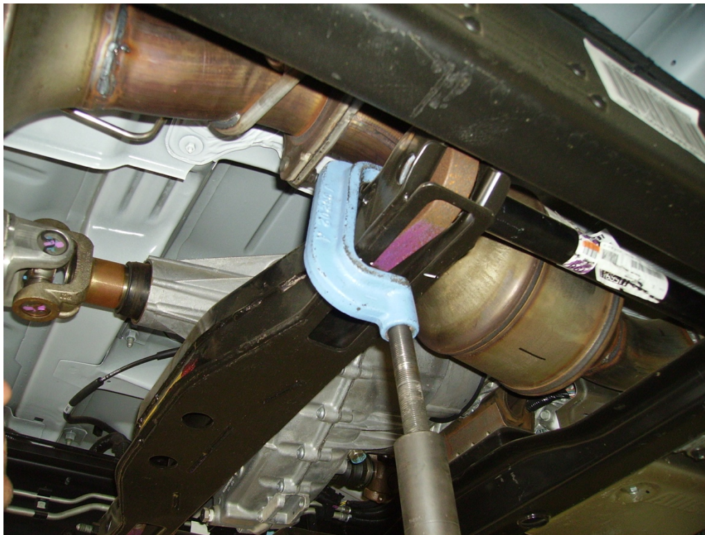
Figure 2: load torsion bar to remove adjuster nut
