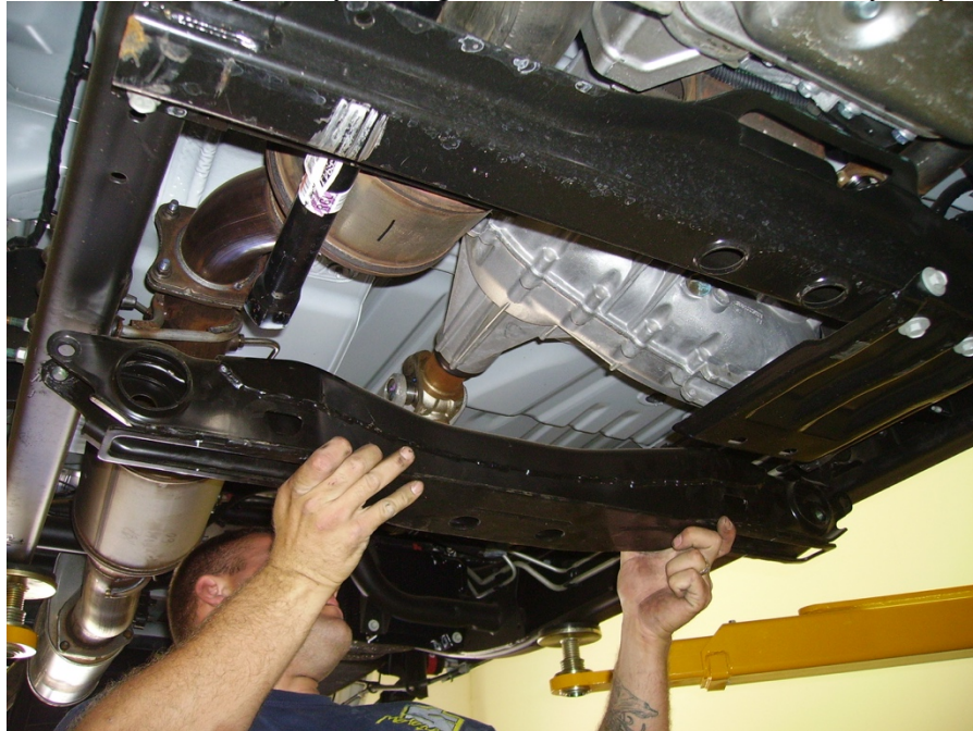
Figure 4: Remove factory torsion bar crossmember
