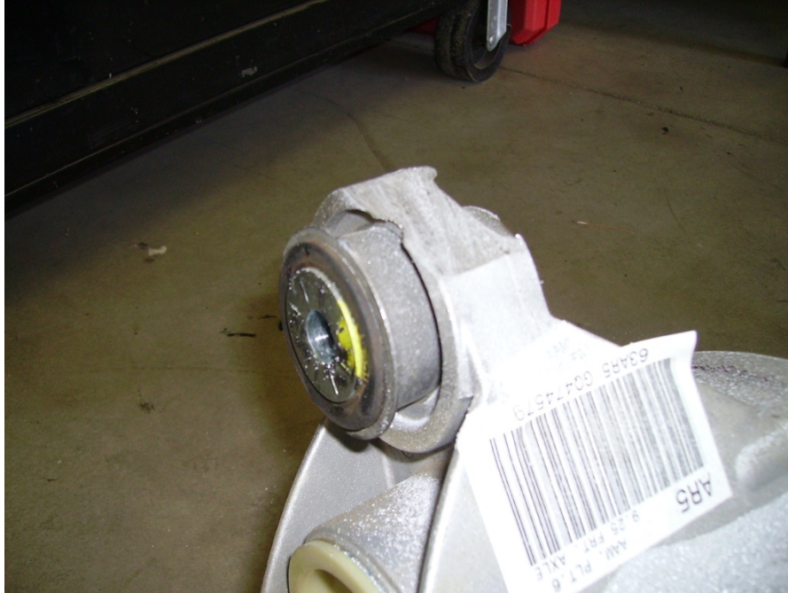
Figure 16: clearance for shoulder nut on pitman arm bracket.
