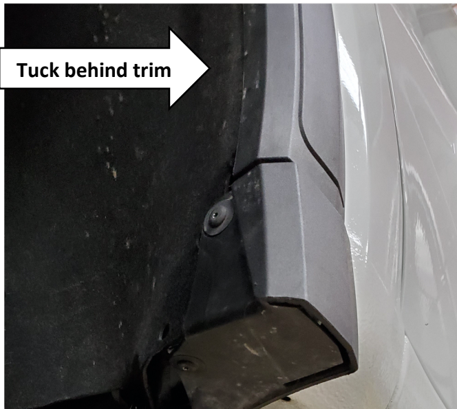
Figure 10: Plastic Mud Flap Trimmed and Reinstalled GMC
