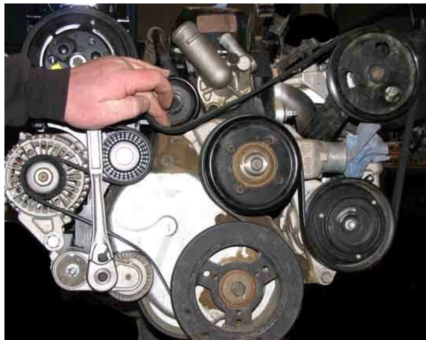
Image 13 Open tensioner and slide belt over edge of upper idler to put in position.
