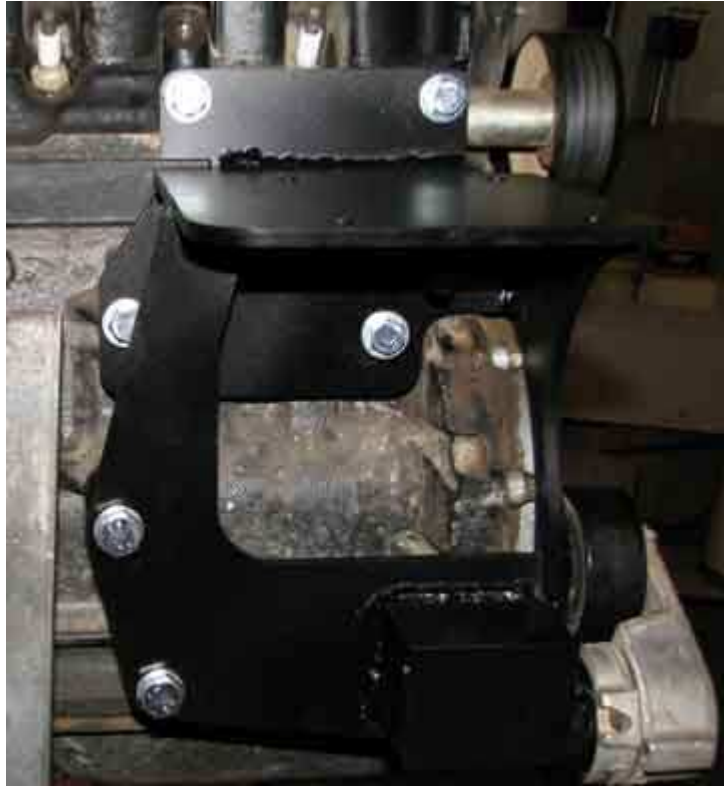
Image 6 Depicting the 6 mounting bolts for the bracket
