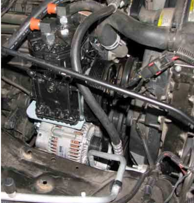
Image 7 York compressor and Alternator installed, you must install the York and tighten the bolts first!
