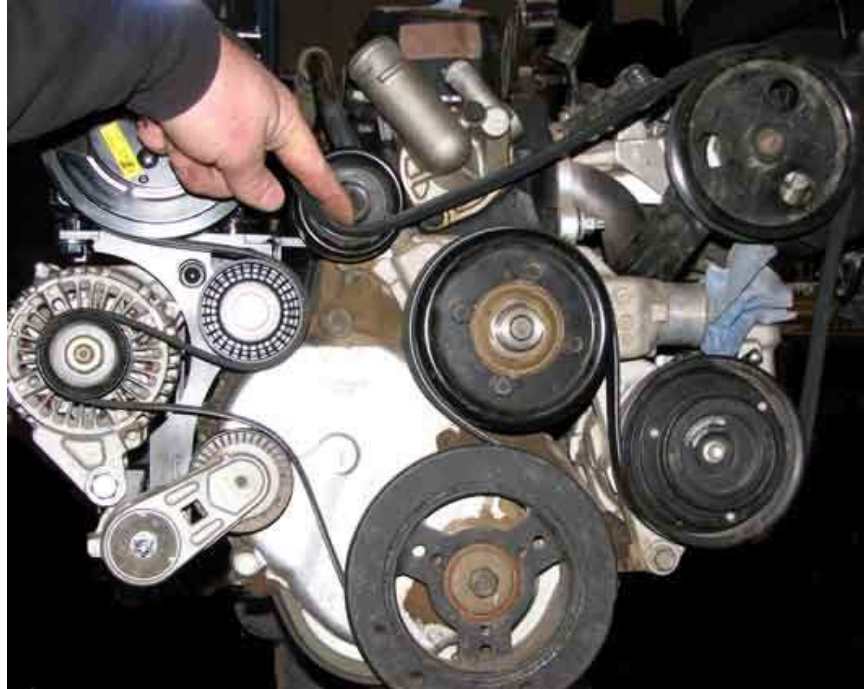
Image 12 Note the belt fully installed other than the top idler
