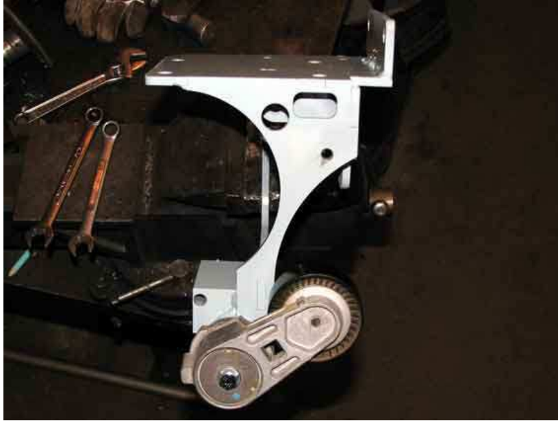
Image 4 Stock tensioner installed on ORO bracket
