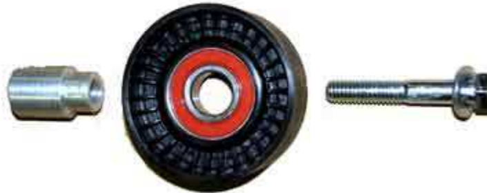
Image 9 Idler pulley, assemble in this direction
