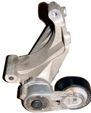
Image 2 OEM Tensioner with torx bolt
