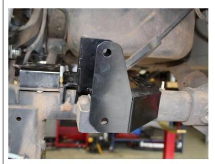
Fit the new rear track bar bracket to the rear axle as shown.
