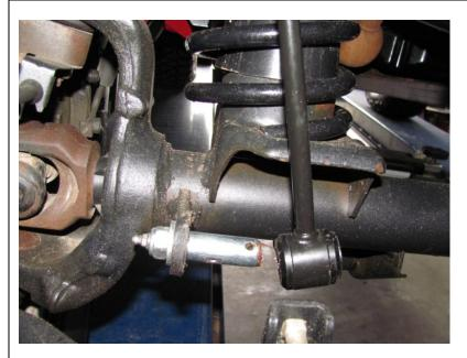
Install new sway bar linkage as shown.
