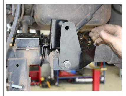
Clamp the track bar bracket in position with the 2 U-bolts provided.
