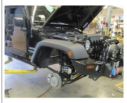
Raise vehicle and support front axle with axle stands.
