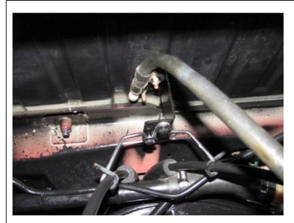
Fit the hand brake relocation bracket as shown.
