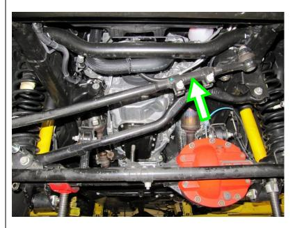
Once axle is centred adjust the drag link to re-centre the steering.
