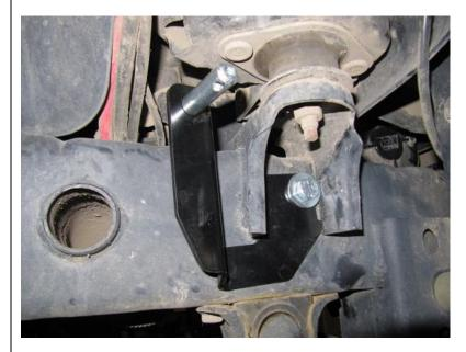
Fit the sway bar disconnect park brackets to the chassis rails.
