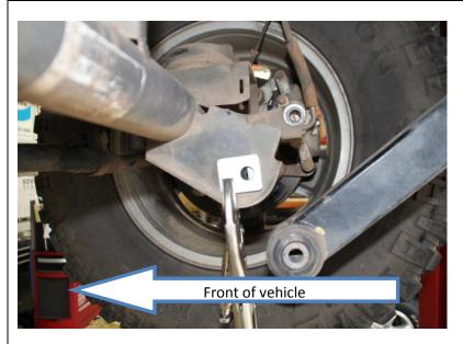
Using vice grips clamp the drive line alignment plates to the axle mount, placing the plates as shown.
