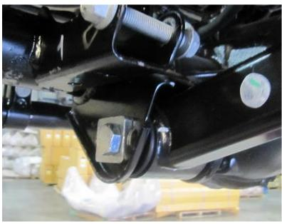
With the alignment plates in position, reconnect the lower control arms using the new M14x110mm flange bolts & cone lock nuts provided.
