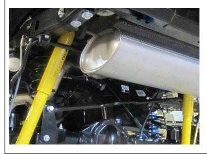
Install new Old Man Emu shock absorbers to top shock absorber mounts using original hardware.
