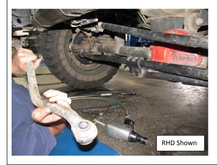
Whilst vehicle is at ride height Remove the front track bar.
