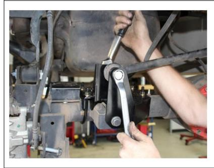
Fit the track bar to the bracket using the new bolt nyloc nut and flat washers provided.
