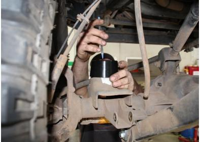
Fit the front bump stop spacers using the fitting instructions provided in the kit
