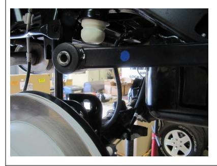
Disconnect the rear upper control arms at the axle end and loosen at the chassis end. Move control arms up, clear of the axle mounts.
