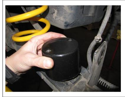
Fit the rear bump stop spacers using the fitting instructions provided in the kit.
