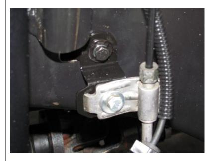
Fit the brake line drop brackets using the fasteners provided as shown.
