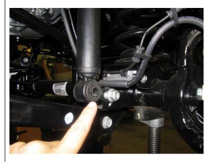
Undo front shock absorber lower mounting bolt and remove front shock absorbers.
