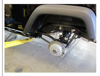
Raise vehicle on hoist and remove rear wheels.
