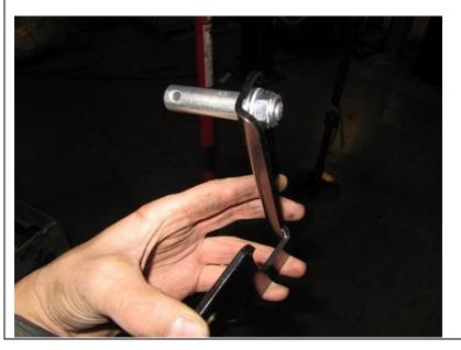
For all models other than Rubicon, a sway bar disconnect system is provided in the kit.
