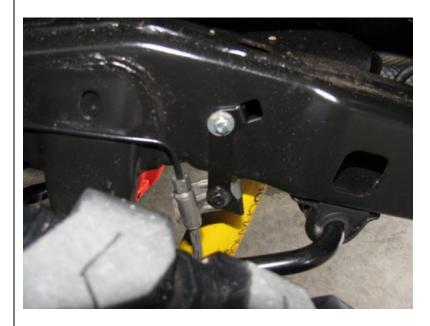
Fit the brake line drop brackets using the fasteners provided as shown.
