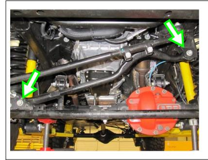
Lower vehicle to ground and fit new Old Man Emu adjustable track bar to vehicle using original bolts.
