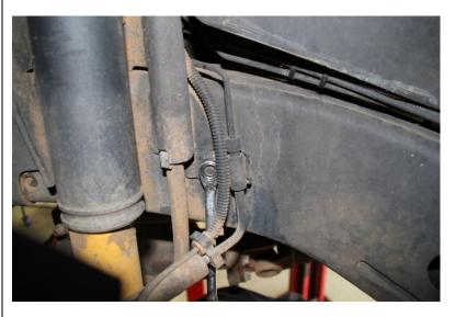
Remove front brake line brackets.
