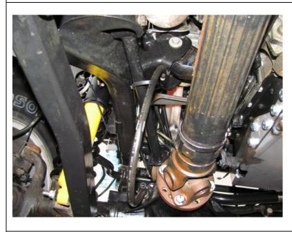
Relocate the front differential breather using a cable tie, as shown, to allow for increased wheel travel.
