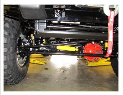
Fit FK50 steering stabiliser relocation kit and new Old Man Emu steering stabiliser.
