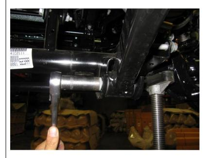
Disconnect the front lower control arms at the axle end and loosen at chassis end.
