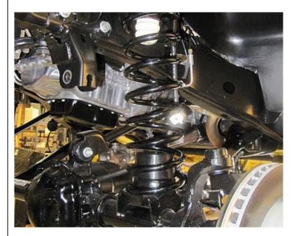
Once the bump stop spacers have been fitted, install the new Old Man Emu springs.
