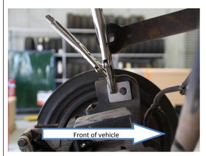
Using vice grips clamp the drive line alignment plates to the axle mount, placing the plates as shown.
