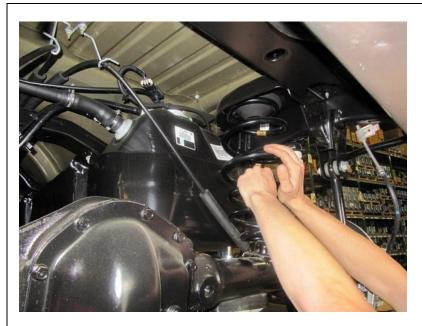
With the bump stop spacers now fitted, install the new Old Man Emu springs.
