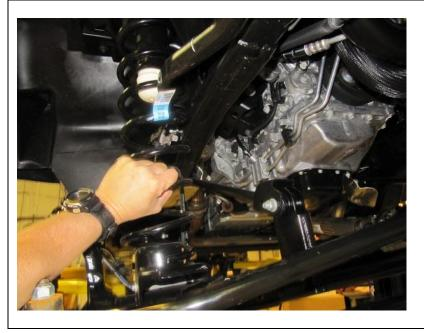
Carefully raise vehicle to remove any load on the front coil springs, so the springs become un-trapped.
