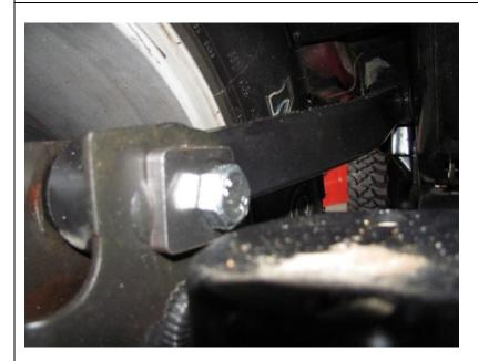
With the alignment plates in position, reconnect the upper control arms using the new M14x100mm flange bolts & cone lock nuts provided.
