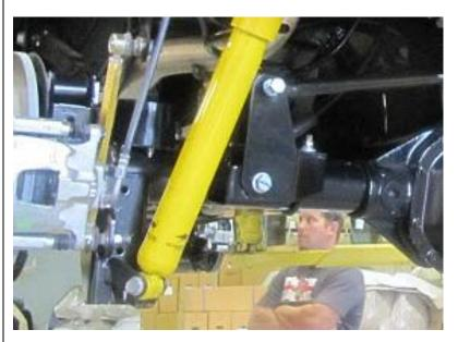
Lower vehicle slightly so that lower shock mounts can be easily reached.
