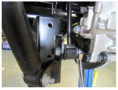
Remove rear sway bar links on both sides of the vehicle.
