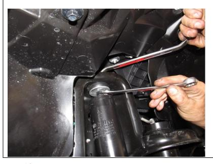
Whilst vehicle is at ride height Remove the top shock absorber mounting nut, washers and bushings.
