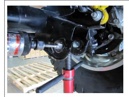
Now the 14mm hole is marked remove the alignment plates.
