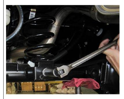
Disconnect the rear track bar at the axle end & back off the torque at the chassis end.
