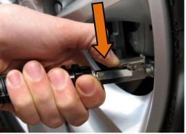
NOTE: ARB's tyre filler attachment is equipped with a stop valve. Air will not pass through the tyre filler attachment until it is connected to a tyre valve.
