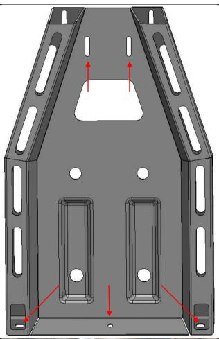
Remove the five M8 bolts locating the transmission panel and remove it from vehicle.
