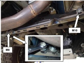
2. Remove rear mount bracket from rear face of transmission cross member using two M8 x 25mm bolts, spring washers and flat washers on the LHS and one M10 SEMS bolt and M10 cage nut and nut plate on the RHS. Replace with new supplied rear mount bracket.
