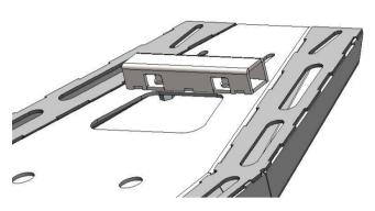
4. Using M8 x 20 bolts, spring washers, flat washers and flange nuts attach spacer to transmission panel.
