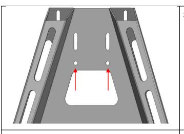
3. Using supplies drilling template (3789203), mark holes, center punch then drill two Ø9mm holes
