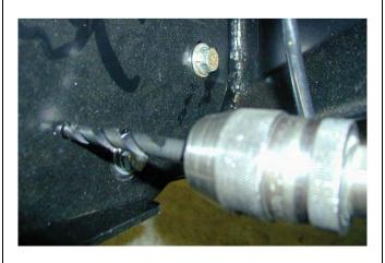
65. With access through light aperture in wing, using the M10 pilot holes in mount brackets (located up 175mm from bottom face of bar), drill pinning hole through uprights on bull bar. Fit M10 screw, washer set and flange nut and do up tight.
