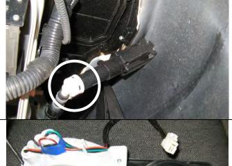
66. If headlight cleaner system to be fitted, reconnect circuit at main joint to vehicle and also hoses to tails of spray heads
