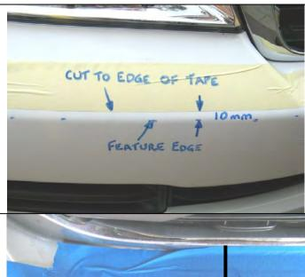
9. Apply wide masking tape edge, carefully aligning 10mm above bumper feature line as shown. Keep the same line level through the centre section of the bumper as shown
