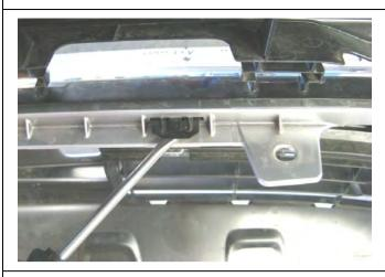
26. Remove grille from bumper cover by releasing plastic tabs as shown
