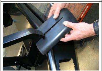
51. Carefully slide top section of buffer past edge of cover strap as shown
