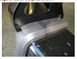
52. Adjust buffers so they sit neatly on the bull bar profile then secure using M6 flange nuts over studs.
