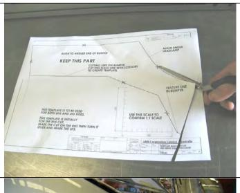
13. Cut A3 paper template along identified cutting line.
