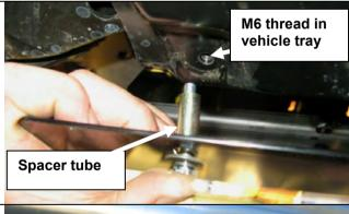
79. Fit stone tray using 4 x M6 bolts and washer sets at front under bull bar and 2 x M6 x 40 bolts, washers and 18mm long tube spacers at two locations into existing sump guard front section as shown.
