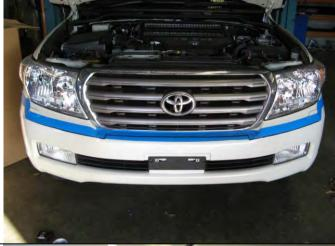
12. Apply approx.200mm of masking tape with edge exactly 90mm from angled bumper end as shown.
