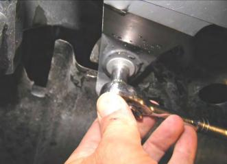
6. Remove lower bumper retaining screws.
