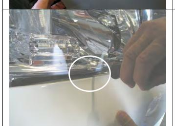
21. Push bumper down immediately below headlamp to gain access with a small flat blade screwdriver and release holding tab.
