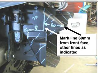
36. Mark the lower section of the air scoop for the power steering radiator as shown. This is for trimming to clear the mount brackets.
