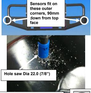
Warning: Cutting operations can result in flying debris, safety
