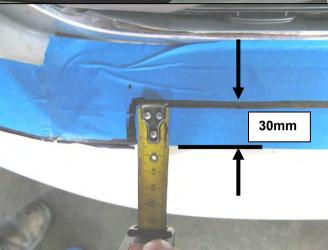
10. Mark out centre cut area of bumper as shown, 740mm wide x 30mm back from feature edge.
