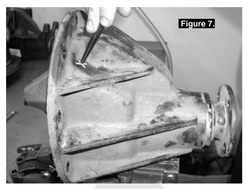
Cover the drive pinion and axle tube areas with a rag to protect them from metal filings.
