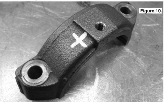
Using a soft jawed vice clamp, setup the bearing cap for drilling the hole at the angle shown (Fig. 11.).
